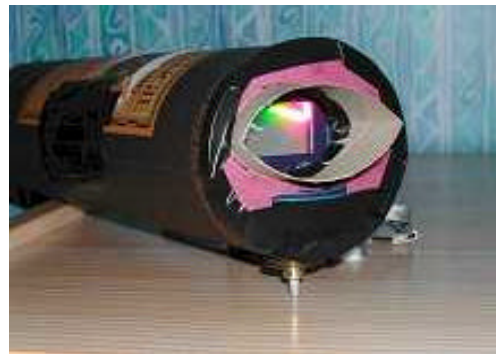
Figure 1: Mark II spectroscope from the viewing end showing the diffraction grating inside
