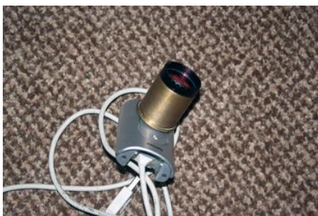
A ToUcam Pro II web camera with adaptor and UV/IR filter attached
