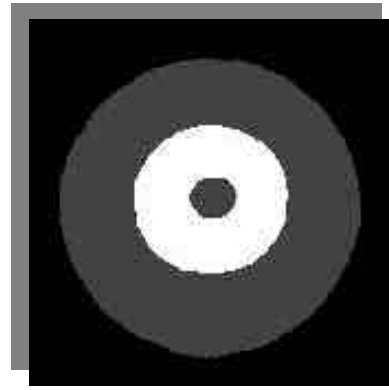
Figure 2: Low power, unfocused star in a telescope that is at least close in collimation.
