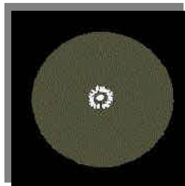
Figure 6: This is what a star might look like in a very high power eyepiece when the telescope is properly collimated
