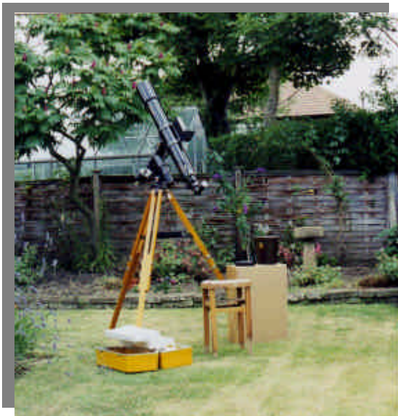
left : 102mm refractor on equatorial mount and wooden tripod
