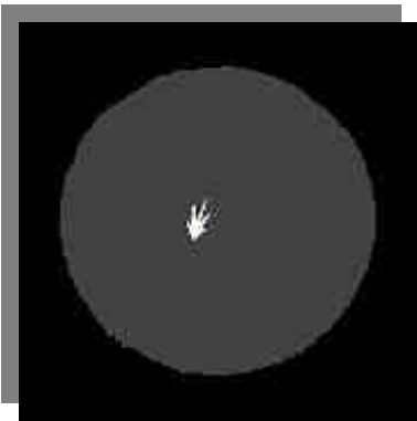
Figure 3: This is what a star might look like in a telescope that is in focus, but not collimated
