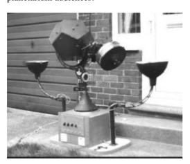
The planetarium will use an A1 Spitz planetarium projector, the first model made by the renowned American company. They are now up to model A5, an example of which has
